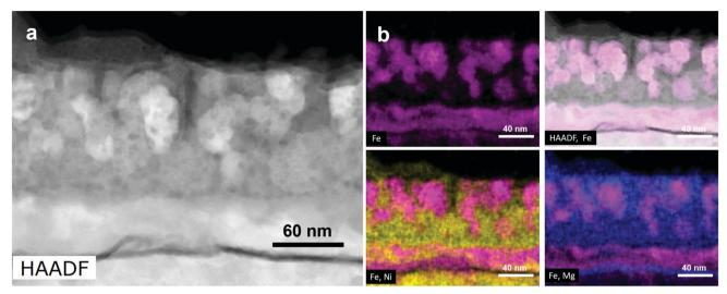
Fig. 1 STEM analysis of Fe-Ni films dealloyed by Mg film at 460 °C for 30 min (\$100-D1) showing the morphology and composition at the dealloying front, indicating formation of Fe and Ni<sub>x</sub>Mg phases from dealloying. (a) High-angle annular dark-field image (HAADF) by STEM, and (b) EDX Analysis of Fe, and HAADF-STEM with Fe, Fe and Ni, Fe and Mg.
