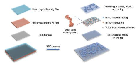
Fig. 5 Schematic of morphological evolution of thin-film-SSID in a Fe-Ni/Mg system
