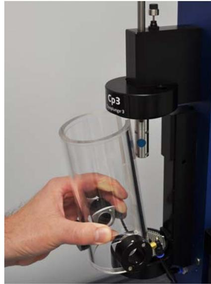
**figure 1-42. Removing the humidity chamber**
