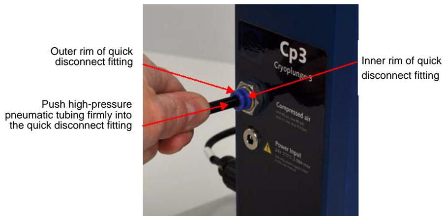
figure 1-8. *Pneumatic connection*
