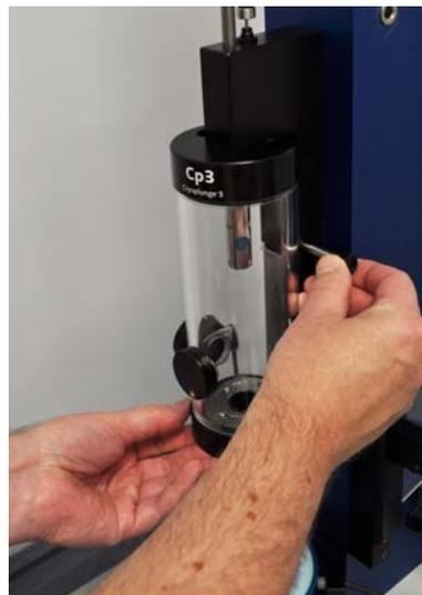
**figure 1-43. Replacing the humidity chamber**
