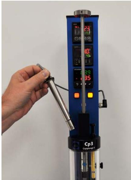
**figure 1-40. Removing the temperature/humidity sensor**
