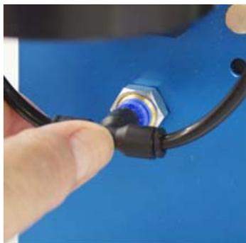
**figure 1-44. Reconnecting the pneumatic supply**
