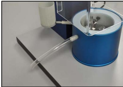
**figure 1-11. Workstation overflow port with Tygon tubing attached**
