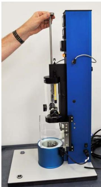
**figure 1-29. Raising the plunge rod to full upward (firing) position**
