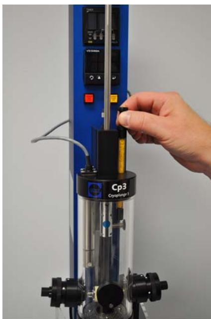
**figure 1-14. Inserting the humidity wand**
