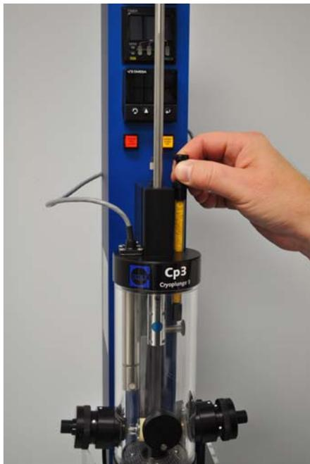
**figure 1-39. Removing the humidity wand**
