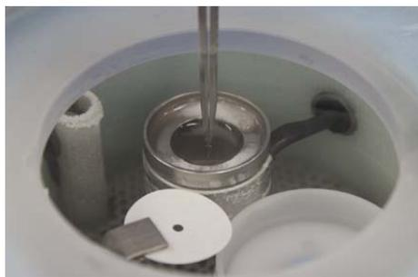
**figure 1-32. Grid plunging into the liquid ethane**
