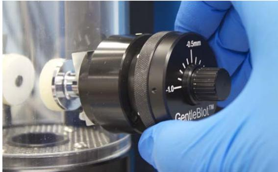
**figure 1-17.** *Inserting/removing a blotter from the right-hand chamber flange*
