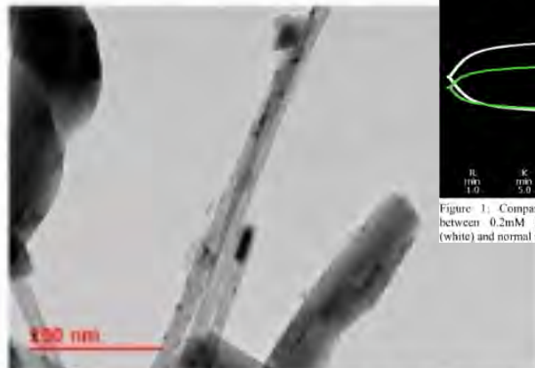
Figure 2: TEM imaging of 3 wt% CoO x /hBN (left) and 1 wt% CuO x /BNNT (right)
