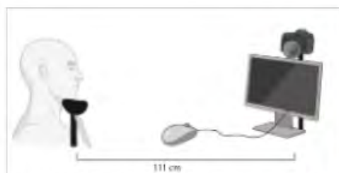
Figure 1: The DISC recording setup. The camera and monitor are located 111 cm away from the chinrest. The participant was instructed to click on Waldo using the mouse. The mirror on the chinrest allows for cross reference of when the Waldo image switches on the monitor, confirming the participant found Waldo.
