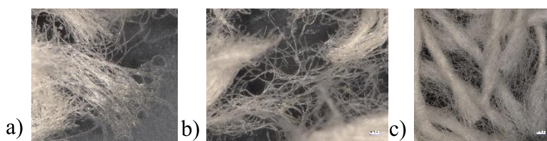
Figure 2: Optical microscopy of deweaved cotton fibers with biopolymer (a), UV-treated biopolymer (b), and water (c).
