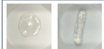
Figure 1: 20% PVA-MA UV crosslinked with Irgacure 651. 3D disk (left), 3D tube (right).
